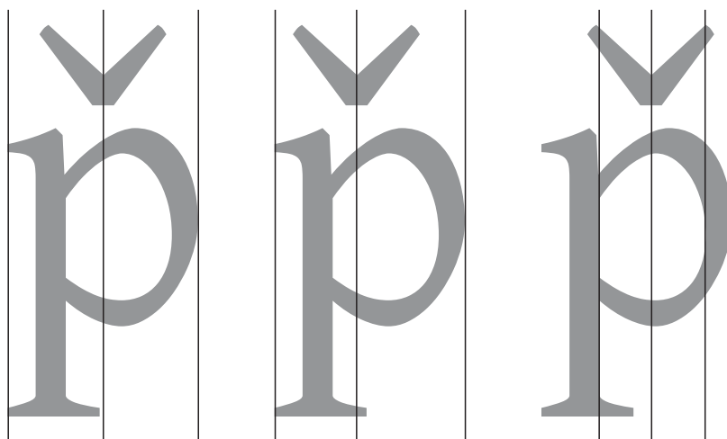
Figure 7. Three different measures of optical centre: the mathematical centre (of the bounding box), the estimated Kindersley optical centre, and the optical centre based upon the counter's Kindersley centre. The mathematical centre may be acceptable, but the normal Kindersley centre is clearly not. The final option gives the best initial alignment, but may need further visual adjustment.
