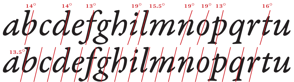
Figure 4.42. Analysis of lowercase slope angles in Garamond Premier Pro Italic Display (top) and Caption (bottom) optical sizes. There is less slope variation in the smaller (caption) size.
